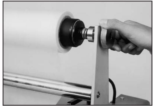
Photo 12A. Loosening tension.
