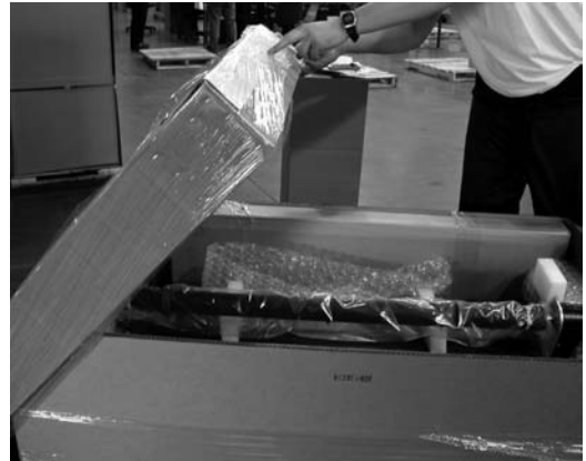
Photo 7B. Remove cardboard box top from laminator skid.
