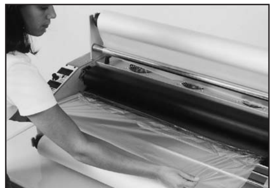
Photo 14C. Grasp the cut film and gently pull as the laminator runs in reverse at a very slow speed.
