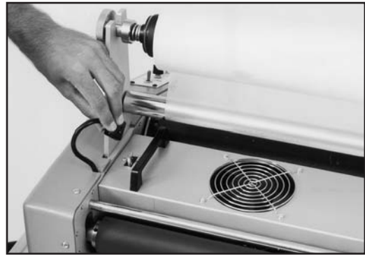
Photo 15A. Cooling fans plug.
