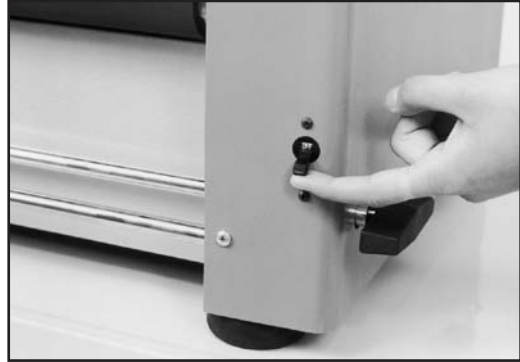
Photo 8A. Turning on the main power switch.
