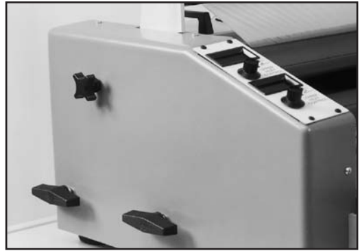
Photo 13A. Roller lift knob adjustments allow for lamination of thicker substrates.
