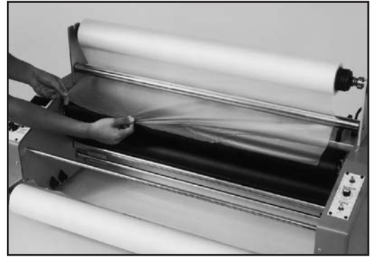
Photo 11A. Thread film around top idler.
