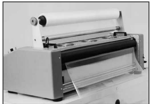
Photo 12B. Clear film exiting laminator after correct tension is applied.
