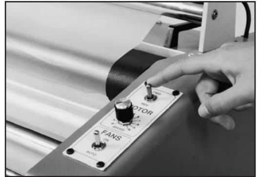
Photo 14A. Automatic reverse switch.
