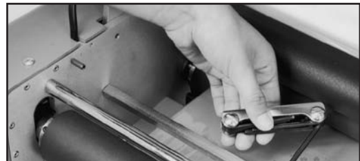
Photo 15C. Using an Allen wrench, loosen the locking screw on the slitter block.
