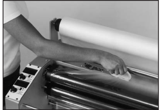
Photo 16A. Cut the film web, leaving approx. 5" of film extended beyond the idler bar.
