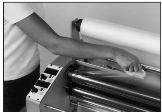
Photo 14B. Cut top and bottom film webs where they wrap around idler bars.
