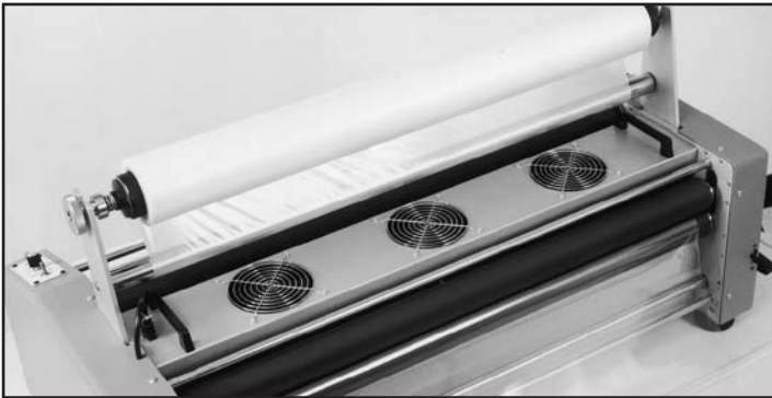
Photo 15B Cooling fans.
