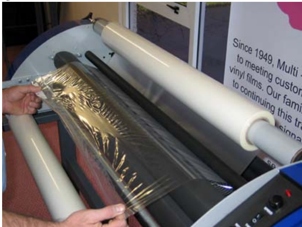
Fig 7.1 POSITIONING TOP WEB
