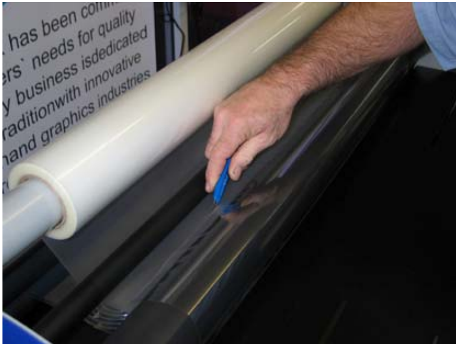
Fig 9.2 CUTTING TOP WEB
