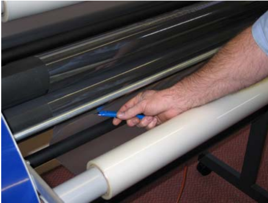
Fig 9.3 CUTTING BOTTOM WEB
