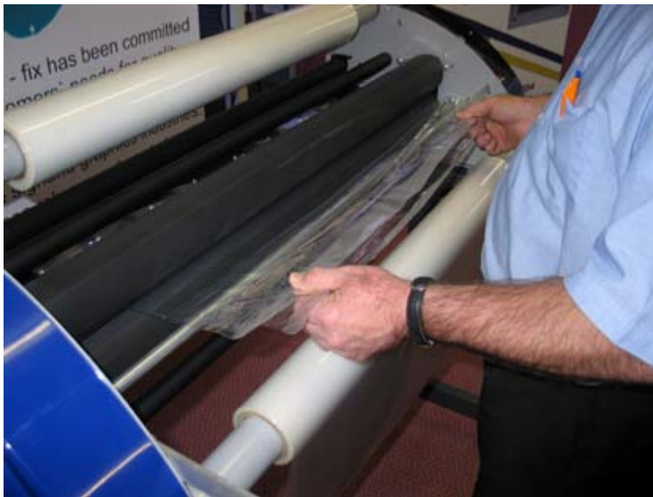
Fig 9.4 REVERSING FILM OUT
