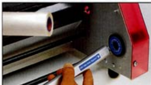
Color Code helps you easily match up the correct side of the roll when installing film onto your roll laminator.
