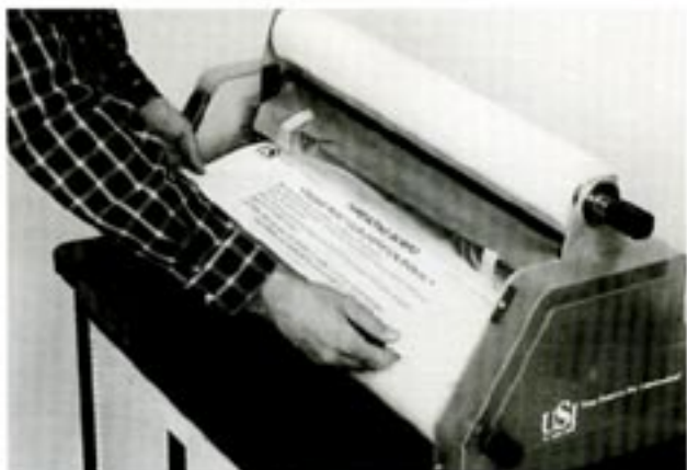
Photo 12-3: Threading board and film web entering.
