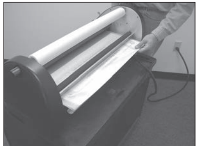
Photo 11-4: Threading board and film web exiting pull rollers.
